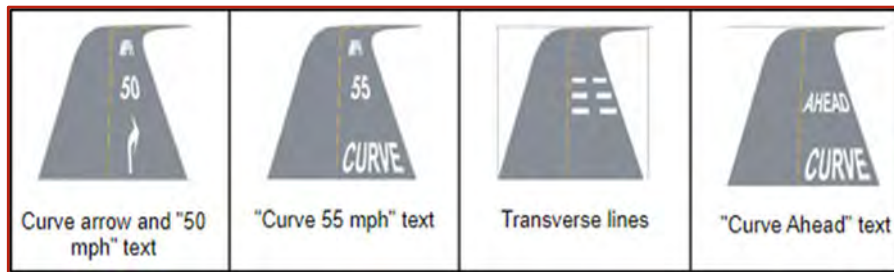
Figure 4-14. Example of In-road Pavement Markings
