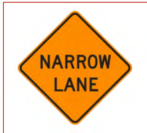
Figure 4-20. MUTCD Sign to Indicate Transition to Narrow Lanes
