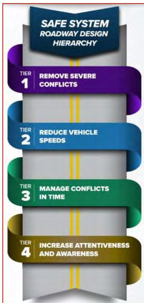
Figure 1-2. Safe System Roadway Design Hierarchy
