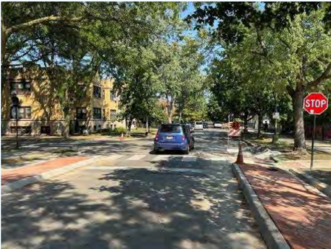
Bump-outs at intersections near the school slow traffic down, improving safety for families walking to school.
