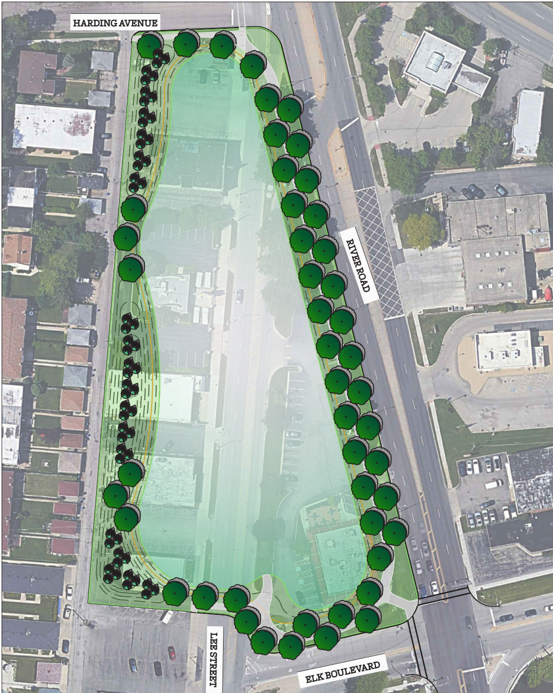
Figure 8.2. Stormwater Concept 4: Lee Street Stormwater Basin
